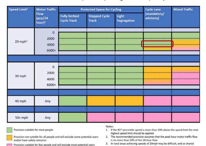
Figure 2: suitability of provision for cycling, as laid out in LTN 1/20, Figure 4.1, "Appropriate protection from motor traffic on highways".
